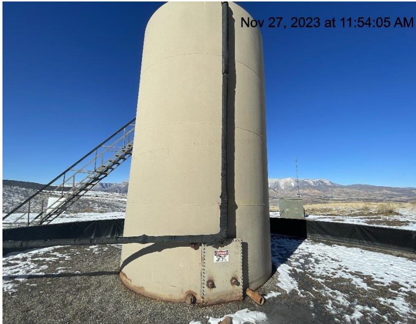
Photo # 7606 Production tank not properly labeled/missing required information
