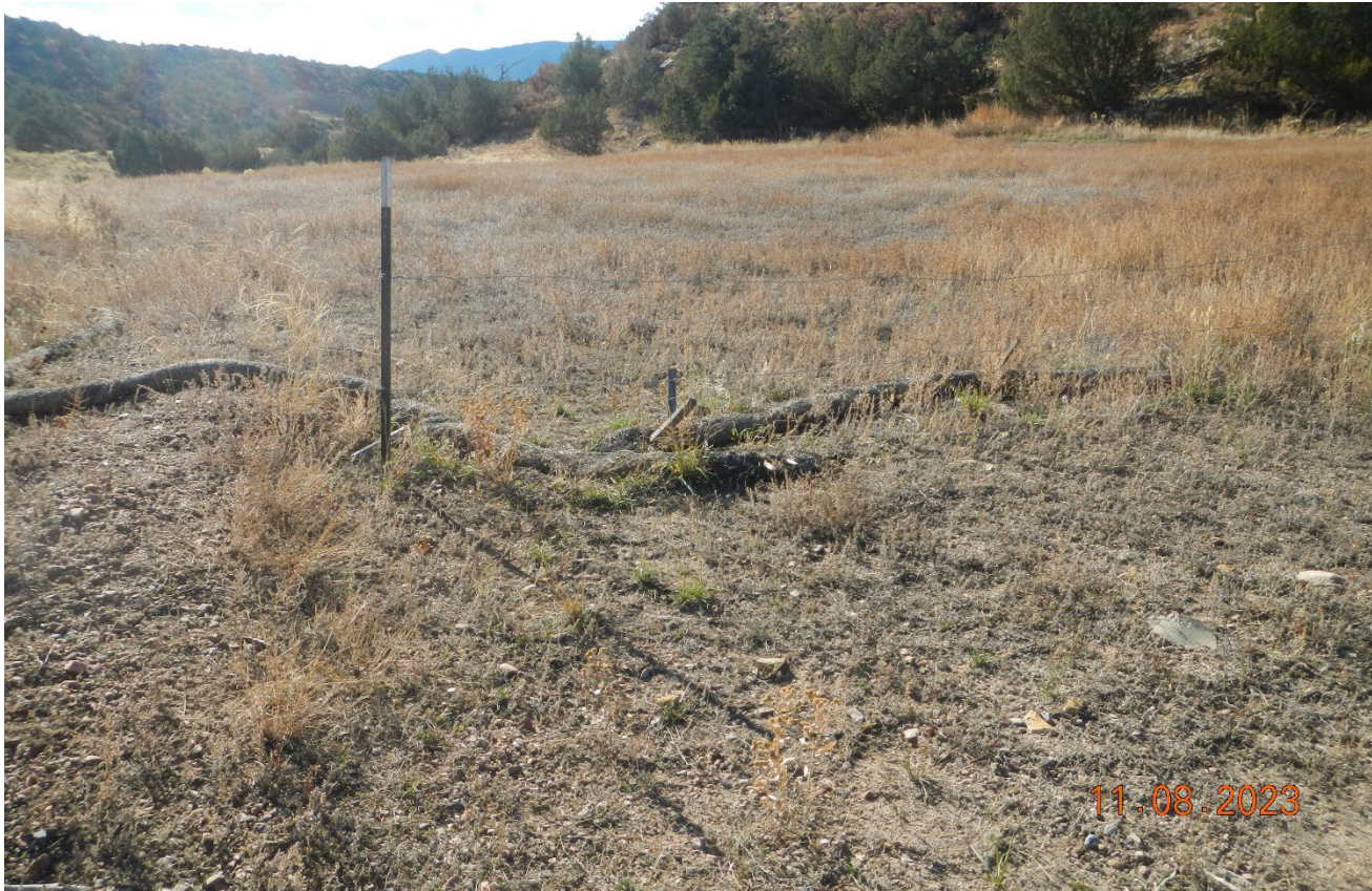
Photo 5. Facing southwest toward the interim reclamation area. There is mostly undesirable weeds growing throughout this area and the straw wattle is displaced. Previous corrective action was not completed.
