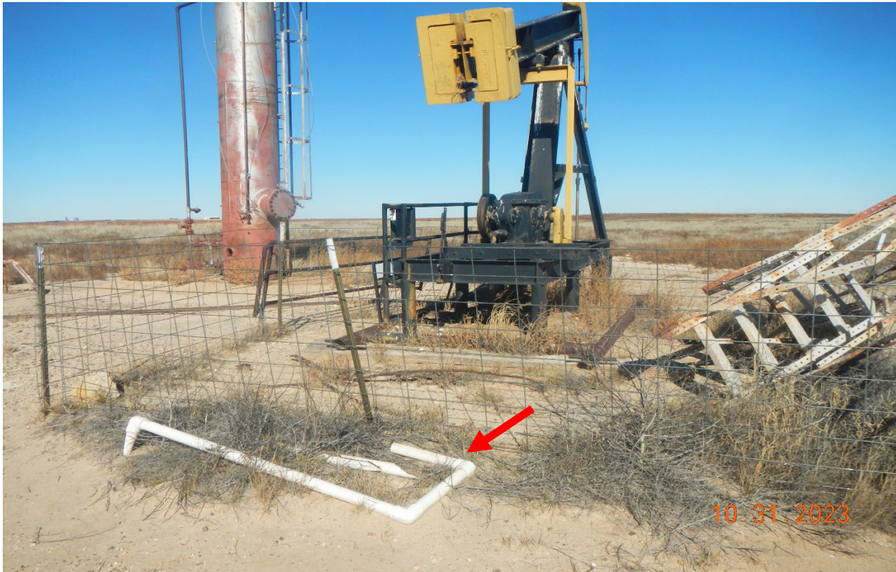
Photo 2. There is a broken pipe at red arrow and weeds around the equipment.
