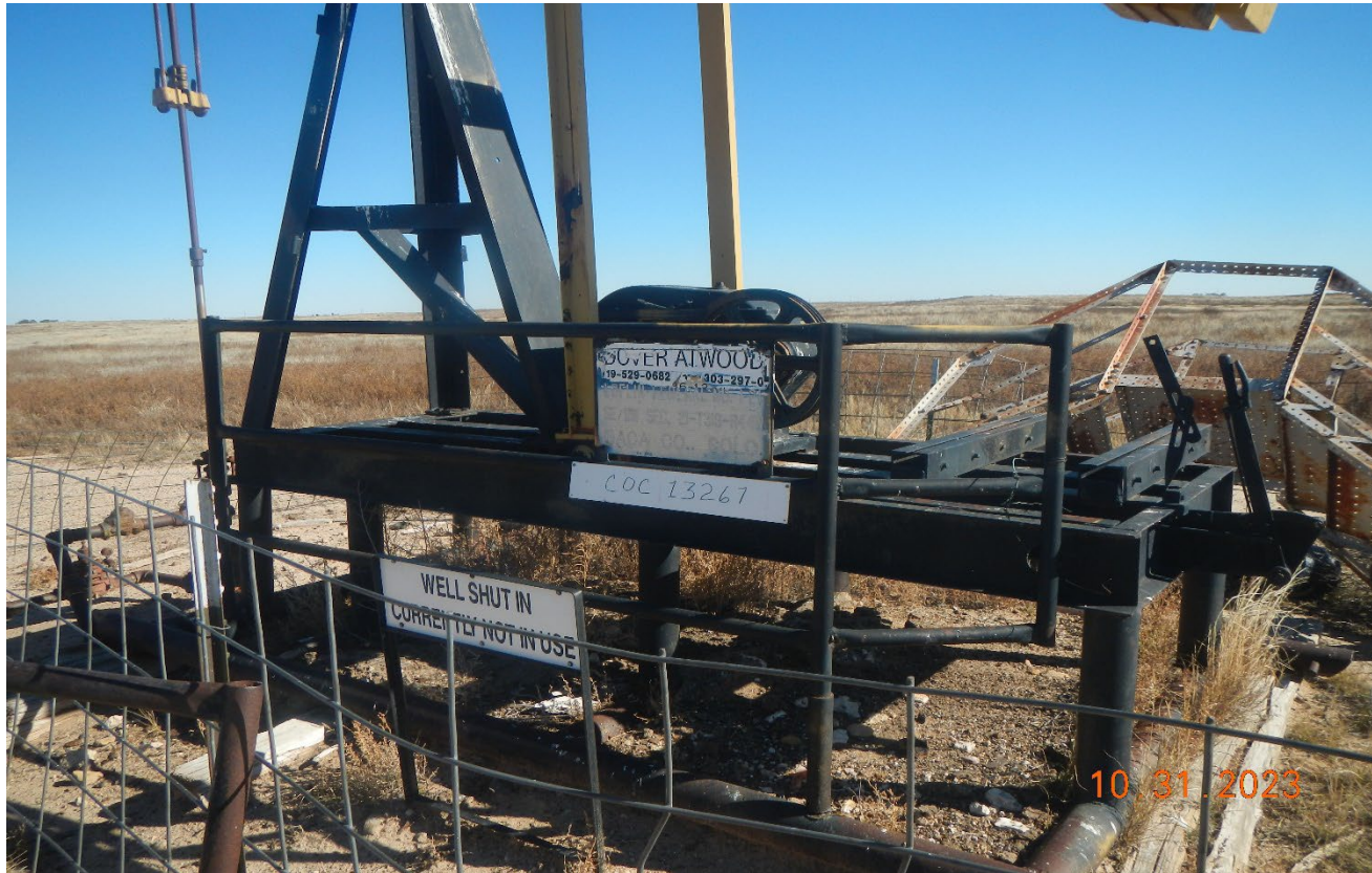
Photo 4. The sign posted at the well is faded and does not meet the requirements.
