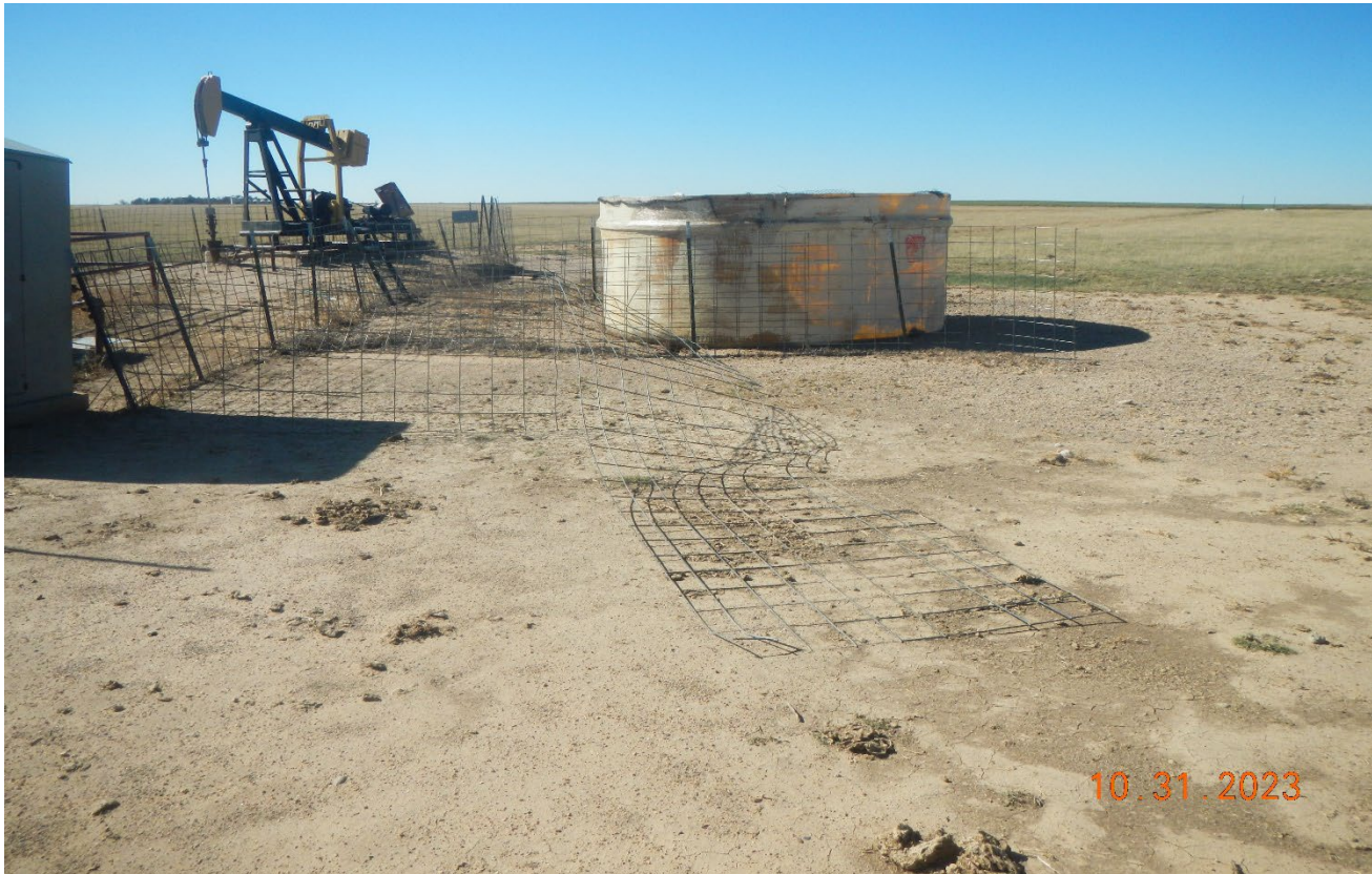
Photo 3. There is no secondary containment around the open top tank. The fence around the equipment is in disrepair and the cattle panel is laying on the ground.
