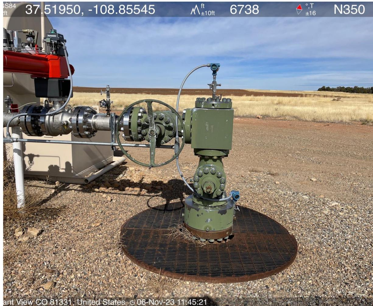
Photo #4 View of the wellhead assembly.
