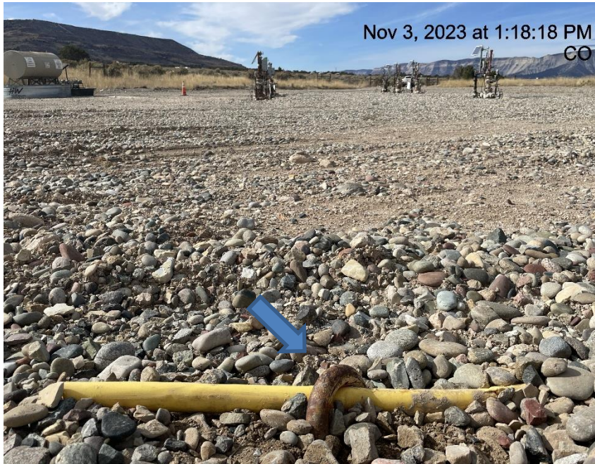
Photo # 5360 Unmarked/improperly marked deadman
