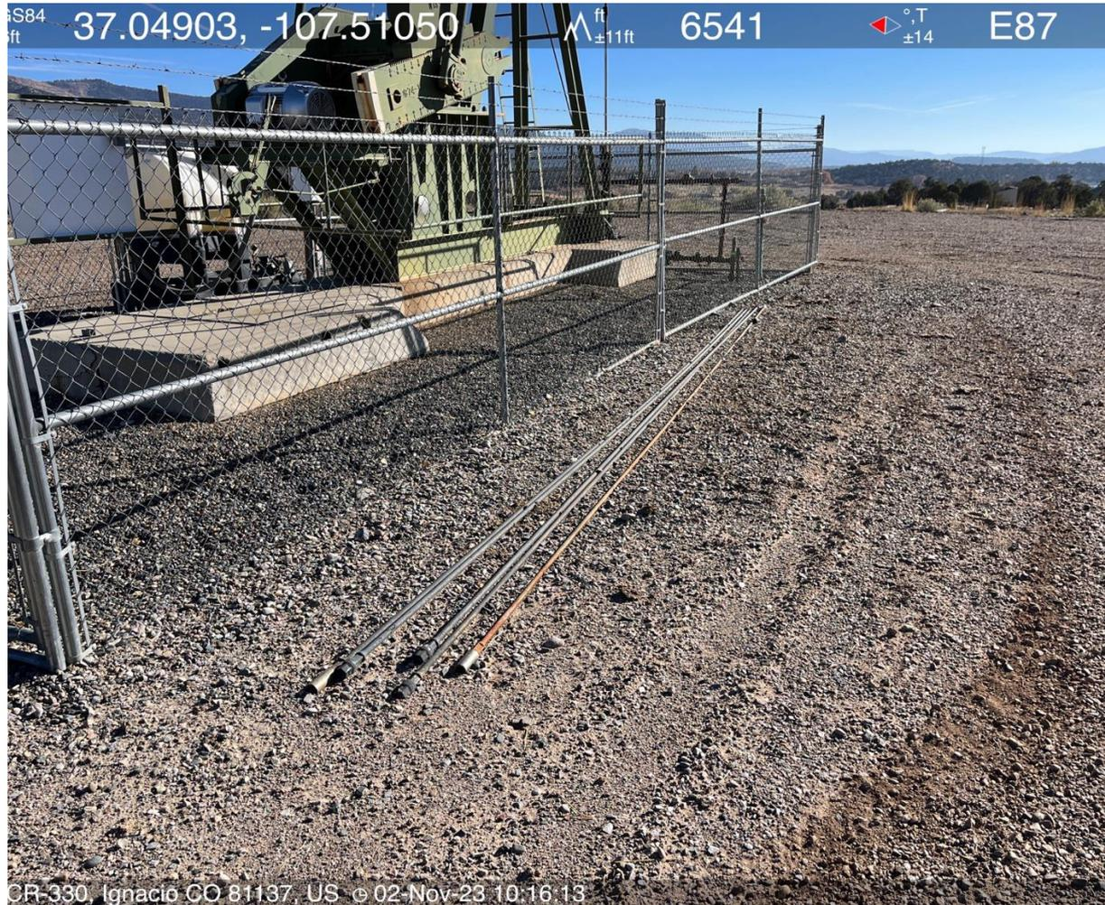
Photo #5 View of sections of sucker rod on ground.
