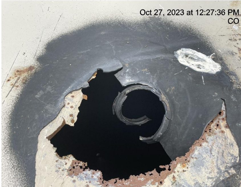
Photo # 4579 Tank has corroded & failed/hole in tank/wildlife hazard
