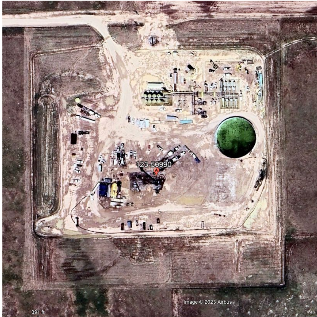
Photo 6. Google Earth aerial imagery from 8/2/2023. Operator has constructed a retention area along the southeastern perimeter; however, a significant amount of stormwater is draining to the southwestern location without sufficient stormwater BMPs.
