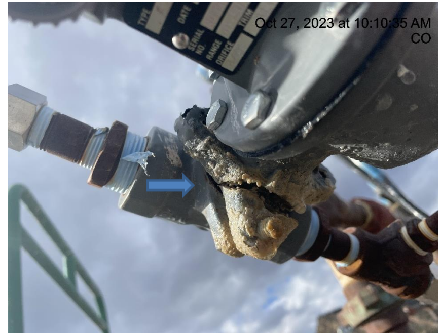
Photo # 4421 Bracket on little joe regulator broken
