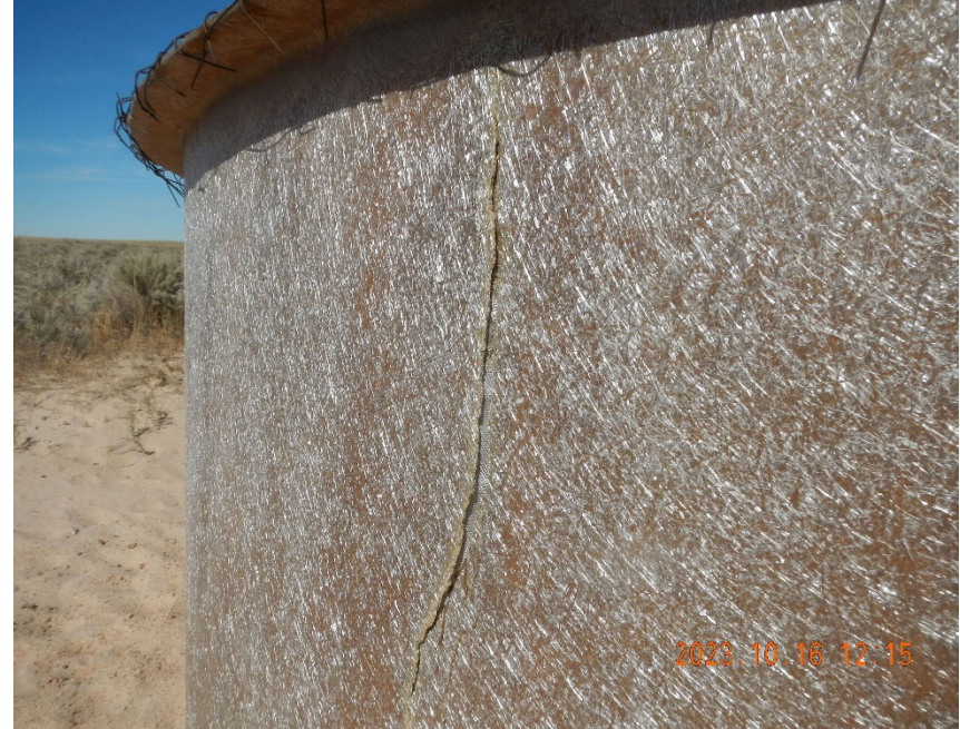
8. Visible split in produced water tank wall.
