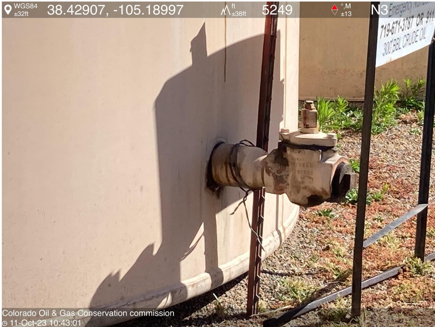
PHOTO 15: Equipment in geologic hazard area not anchored or inadequately anchored. Anchor equipment ensuring anchors are (engineered) to ensure the equipment will resist flotation, collapse, lateral movement, or subsidence per Rule 607. THIS IS THE SECOND NOTICE FOR THIS CORRECTIVE ACTION, IMMEDIATE ACTION IS REQUIRED. NOTE: PER RULE ANCHORING MUST BE ENGINEERED.
