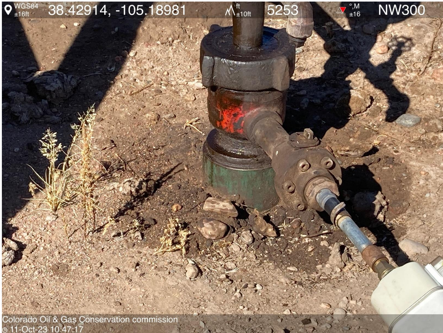
PHOTO 6: AREA OF IMPACTED SOIL AROUND WELLHEAD APPEARS TO BE FROM LEAKING POLISH ROD PACKING. Conduct maintenance on equipment, cleanup stained material and review self inspection processes. COMPLY WITH RULE 1002,(2).D. CA DATE 11-11-2023.
