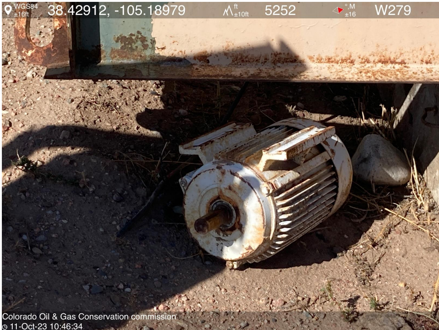
PHOTO 5: UNUSED EQUIPEMNT STORED ON LOCATION (ELECTRIC DRIVE MOTOR NEAR PUMP JACK). REMOVE UNUSED EQUIPMENT PER RULE 606. CA DATE 11-11-2023.
