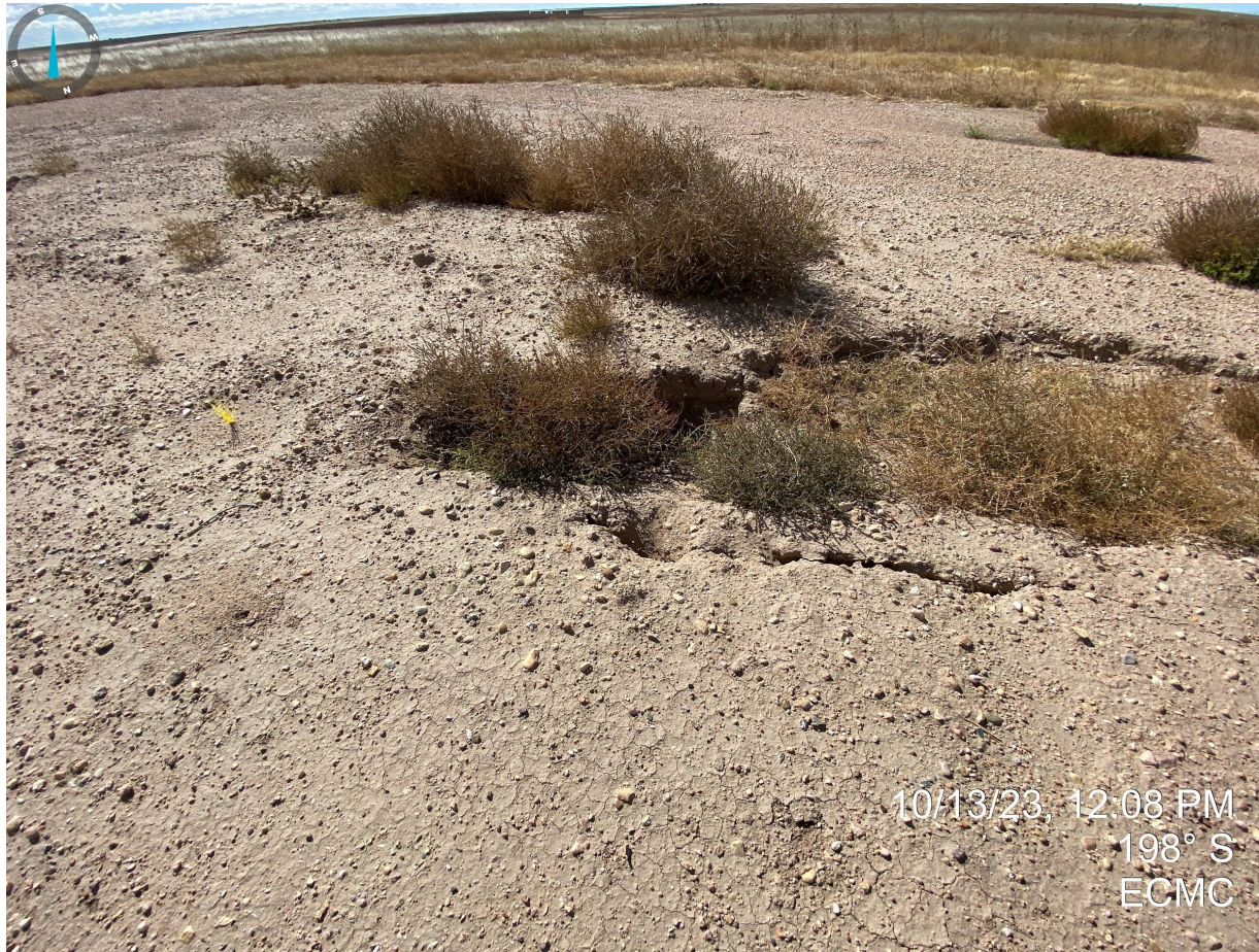
Photo 5. Taken near the former well. Subsidence/hole was observed. The Operator was immediately contacted and instructed to mark/cover the opening to ensure safe operations.
