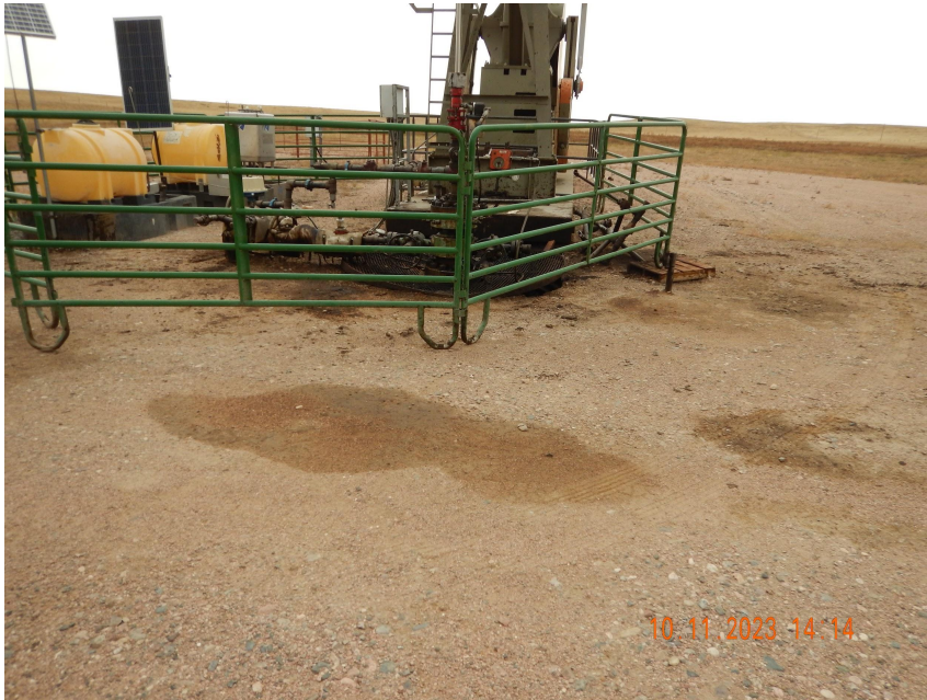
Photo 5. Photo taken from the wellhead. Photo illustrates stained soil around the wellhead and outside of the cattle guards.
