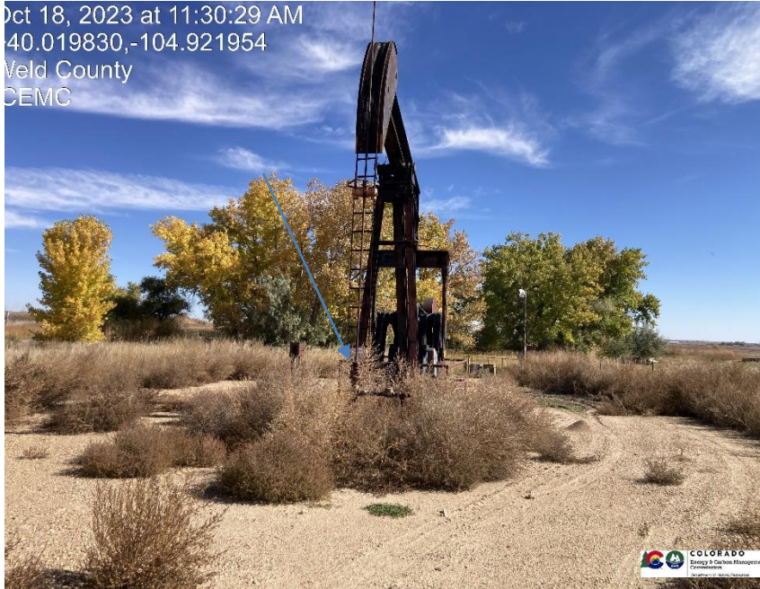
Pic 1 wellhead / pump jack / weeds unmanaged / wellhead sign has fallen off of pump jack and needs to be replaced.
