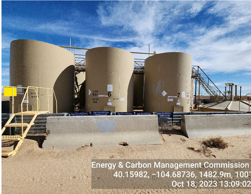
Photo 5: Centralized tank battery
