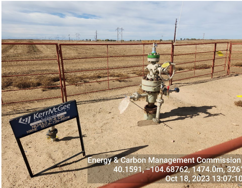
Photo 3: TA Wellhead
