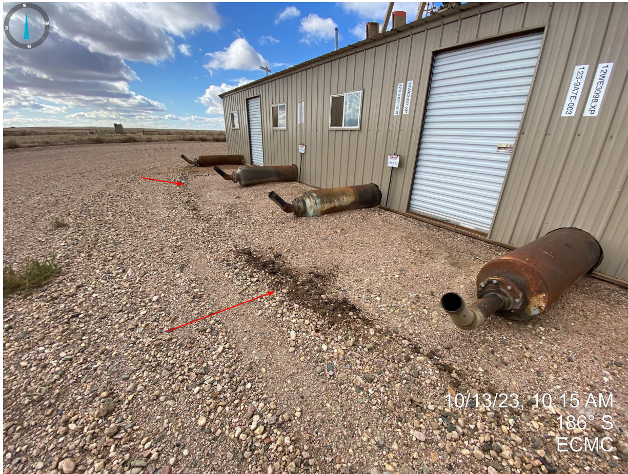
Photo 6. Stained soils observed near pump jack mufflers.
