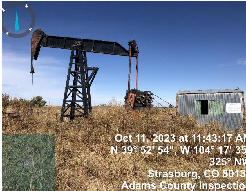
Photo#1 Pumpjack/Wellhead
