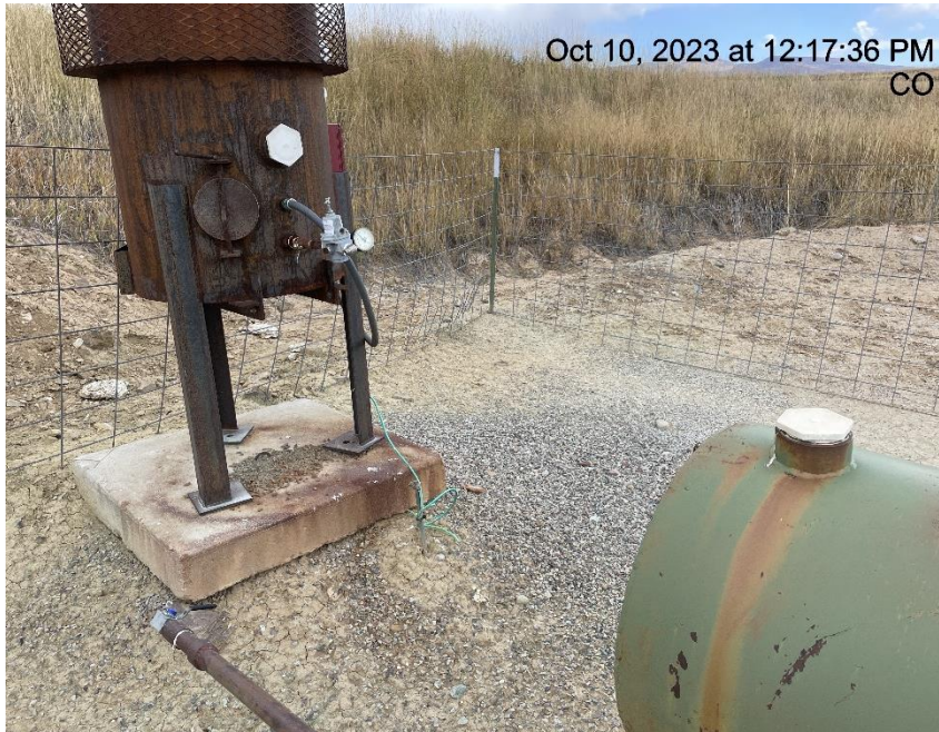
Photo # 2297 Unused equipment/ECD is disconnected
