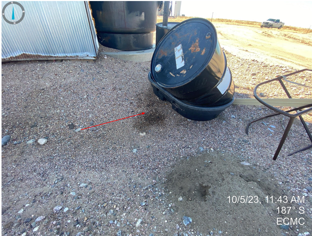
Photo 4. Stained soil observed near drum without adequate secondary containment.
