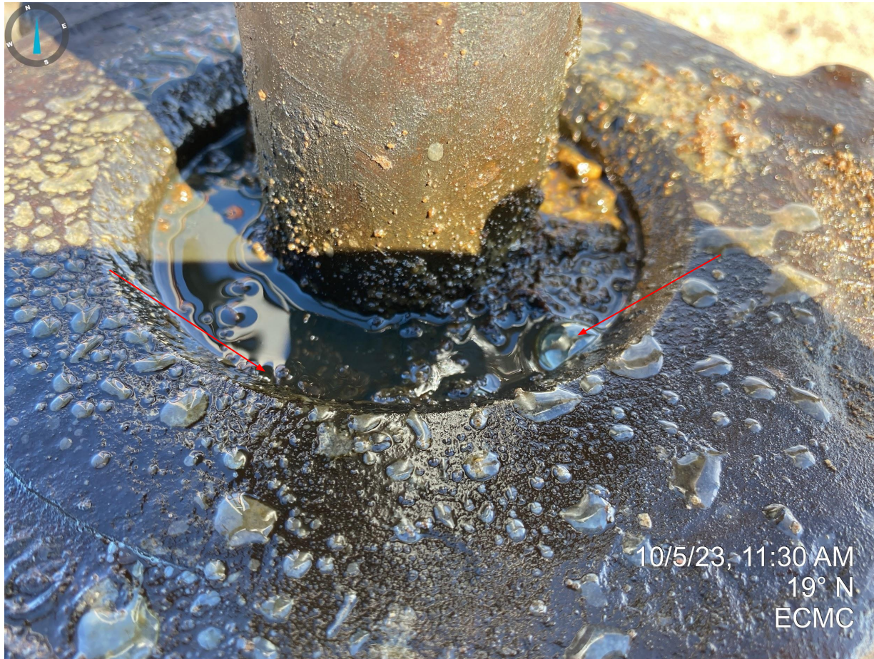
Photo 18. Audible and visual leak detected at wellhead/stuffing box hammer union.
