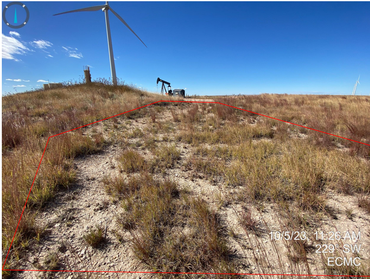
Photo 12. North of the location, within the interim area. Non-uniform vegetation cover resulting in areas of bare/exposed soils.
