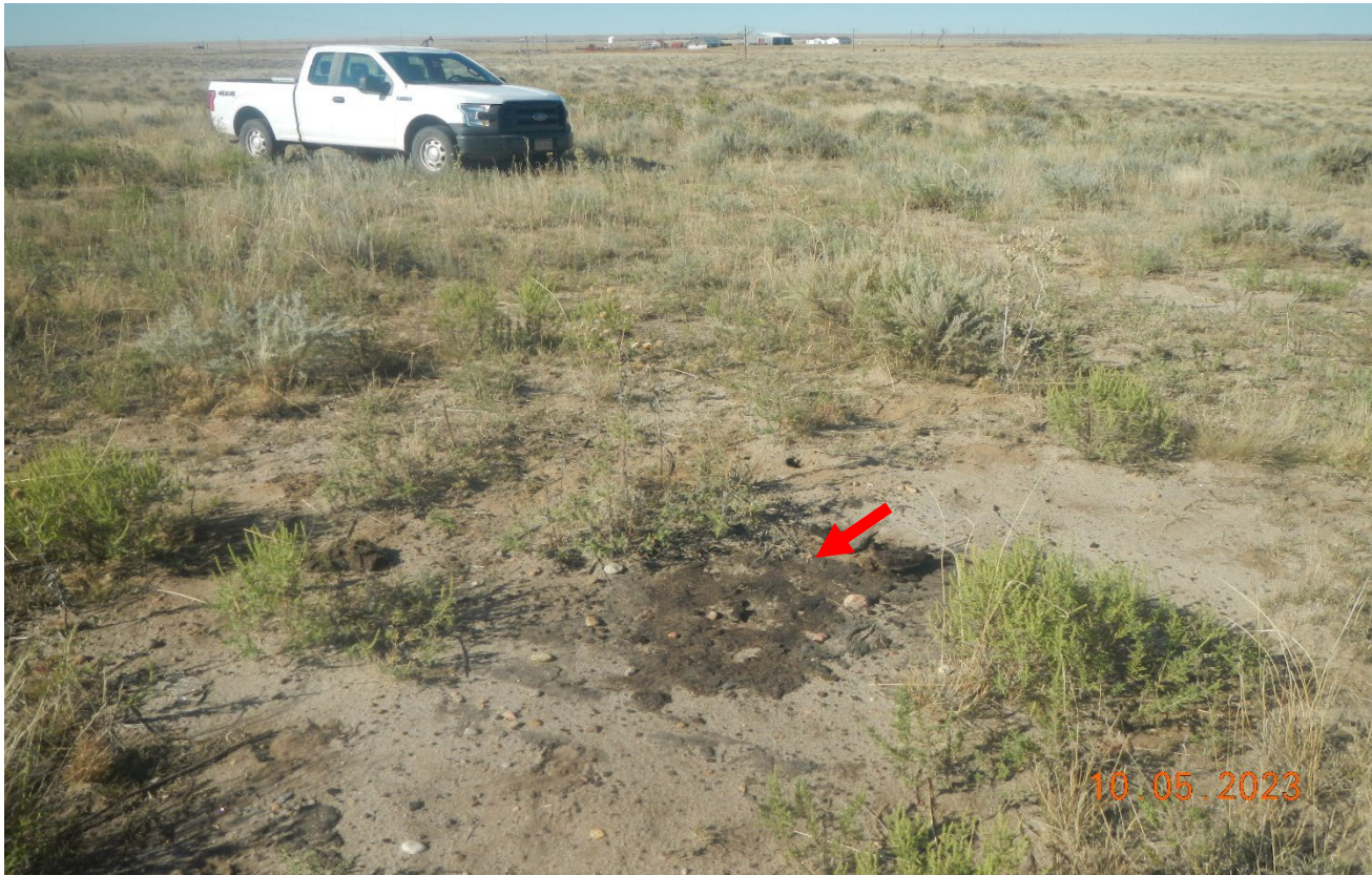
Photo 4. Facing southwest along the abandoned flowline near the location. There is oily sludge shown at red arrow that needs to be cleaned up. Lat/Long:38.42686,-102.46158.
