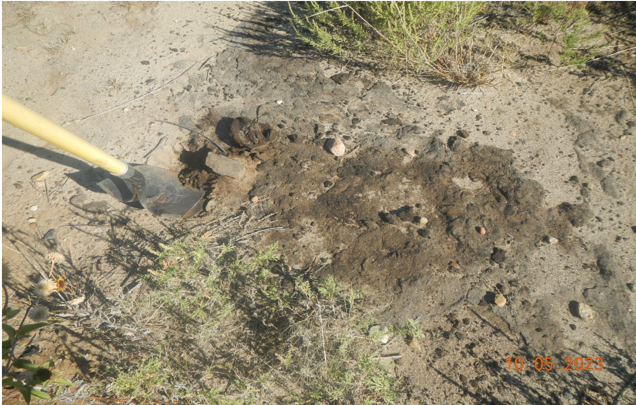
Photo 2. View of oily sludge shown at the surface. Lat/Long:38.42686,-102.46158.
