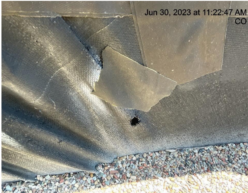
Photo # 2280 From inspection 708900904 conducted on 06/30/2023 Hole in secondary containment liner/liner needs maintenance
