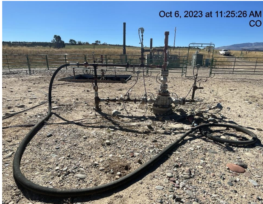
Photo # 1916 KELLY 34-13 well bradenhead connected to flowline
