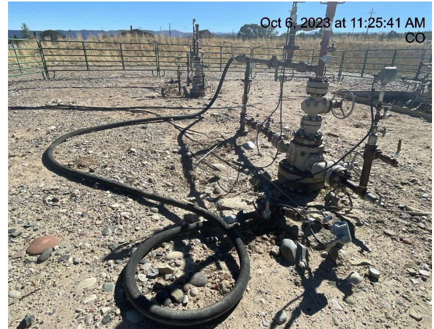
Photo # 1917 KELLY 34-13 well bradenhead connected to flowline
