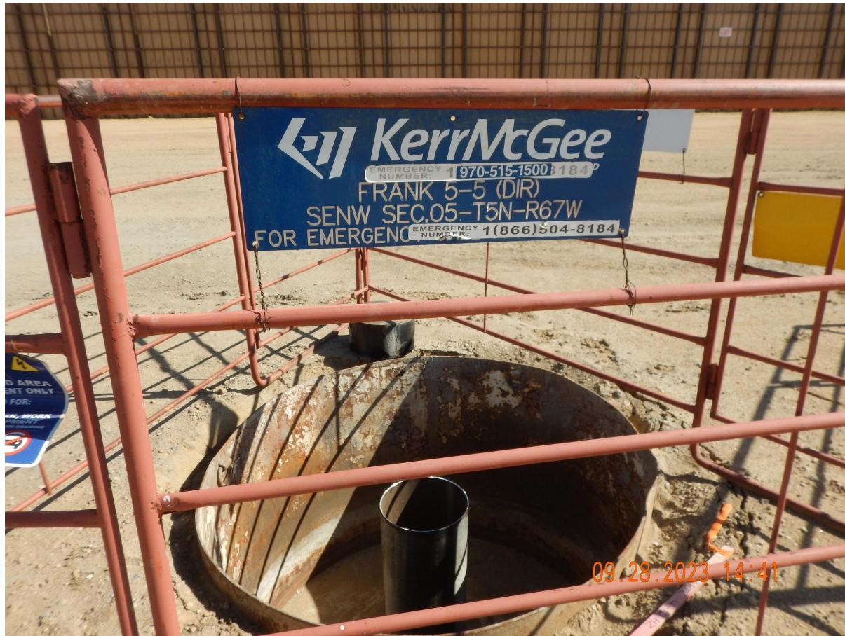
Photo 12. Photo illustrates there is no night cap on surface casing. Operator shall comply with Rule 406.e.(1) and follow their own BMP from the Wildlife Mitigation Plan.
