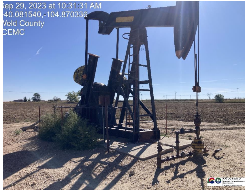
Pic 1 wellhead / pump jack
