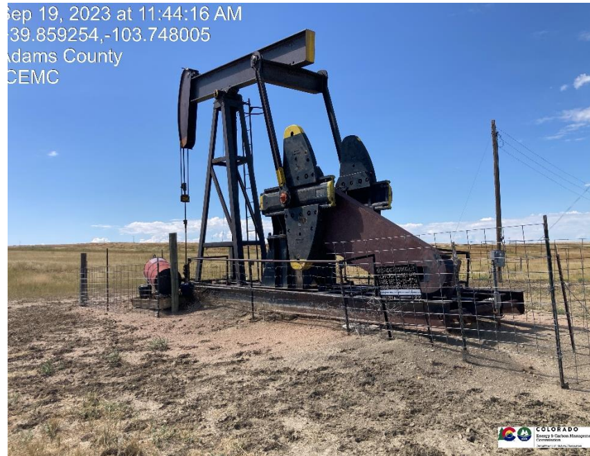
Pic 1 wellhead / pump jack
