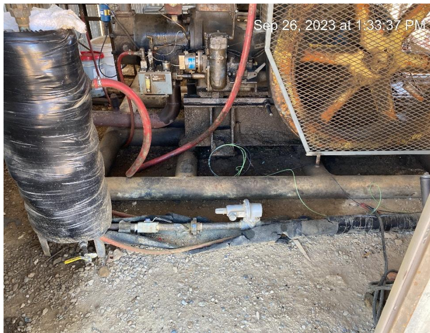
Leaks and staining sill remain as in previous inspection
