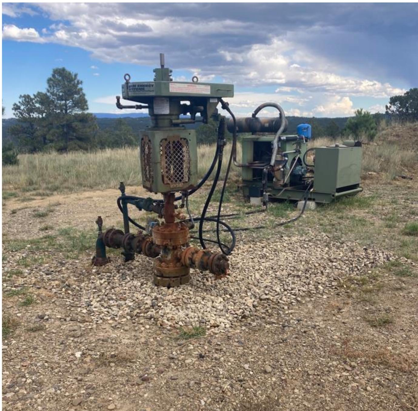
PHOTO 1: THE HYDRAULIC LEAK WAS REPAIRED AND EQUIPMENT MAINTENANCE HAS BEEN PERFORMED. ALL IMPACTED SOIL WAS REMOVED FROM THE LOCATION AND FRESH PAD MATERIAL ADDED AROUND THE WELLHEAD. THE SELF INSPECTION PROCESS HAS BEEN REVIEWED.
