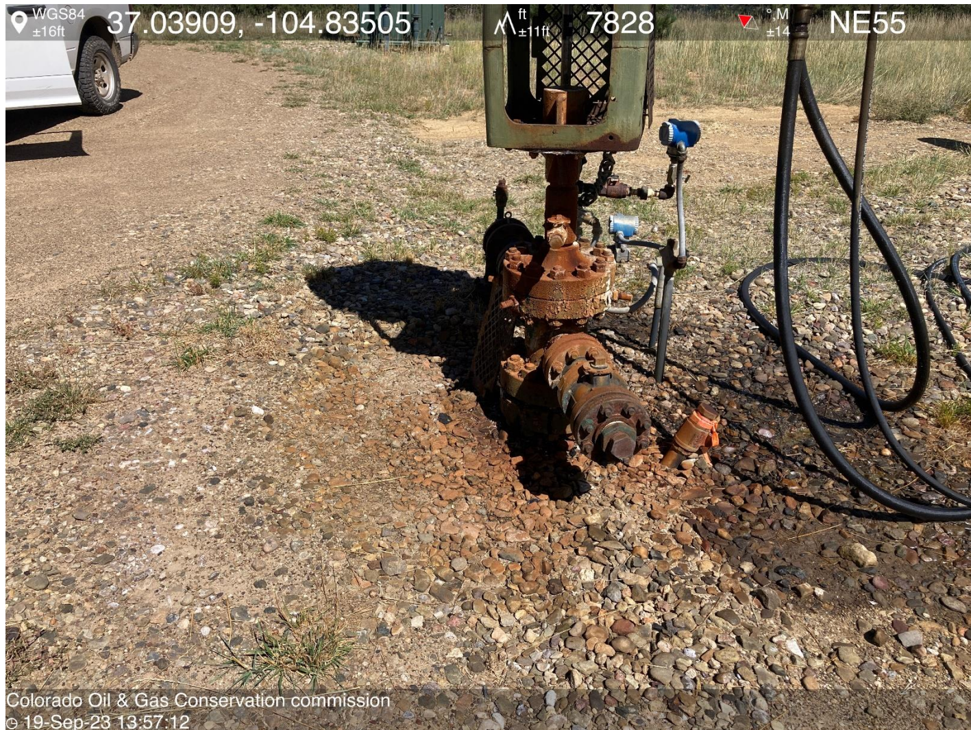
PHOTO 6: RUST COLORED IMPACTED SOIL APPEARS TO BE FROM ROD PACKING LEAKING OVER MULTIPLE EVENTS. Conduct maintenance on equipment, cleanup stained material and review self inspection processes. COMPLY WITH RULE 1002,(2).D. CA DATE 9-30-2023.
