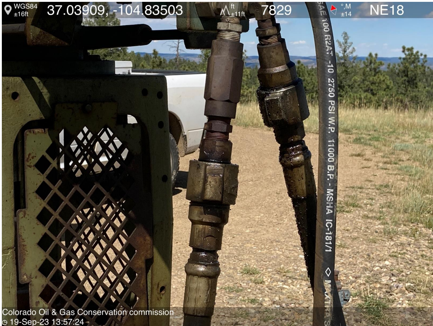
PHOTO 4: QUICK CONNECTIONS ON DYDRO HOSES ARE LEAKING. Conduct maintenance on equipment, cleanup stained material and review self inspection processes. COMPLY WITH RULE 1002,(2).D. CA DATE 9-30-2023.
