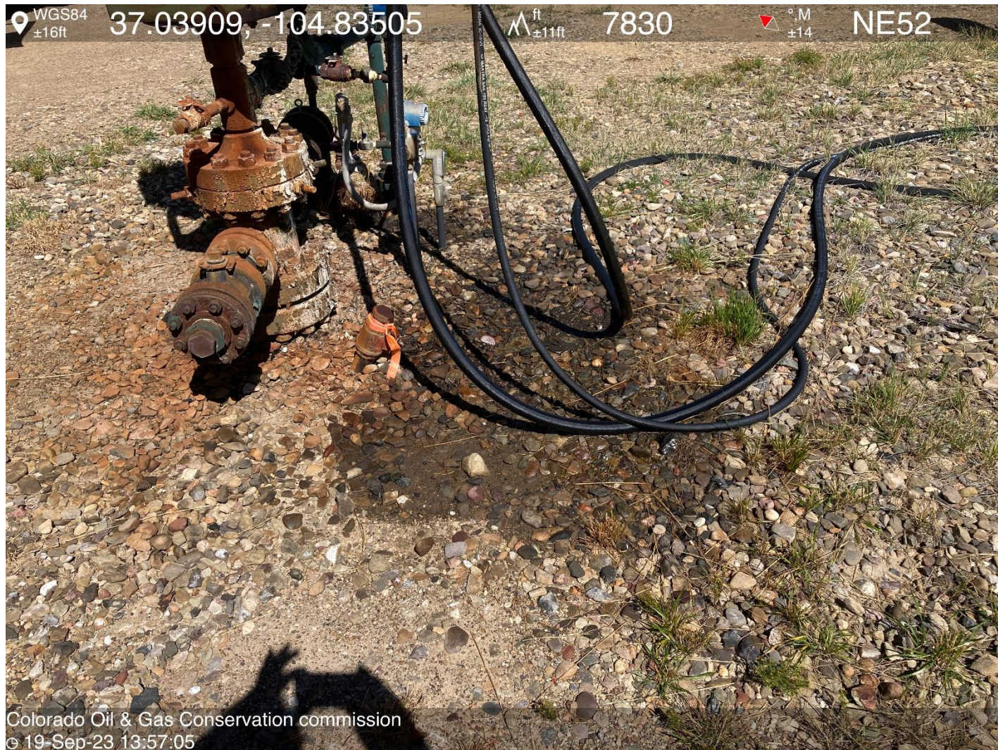
PHOTO 5: AREA OF IMPACTED SOIL UNDER DYDRO QUICK CONNECT HOSED. Conduct maintenance on equipment, cleanup stained material and review self inspection processes. COMPLY WITH RULE 1002,(2).D. CA DATE 9-30-2023.
