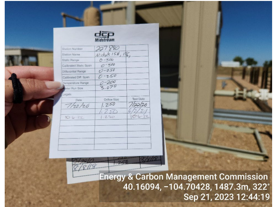
Photo 10: Gas meter not annually calibrated
