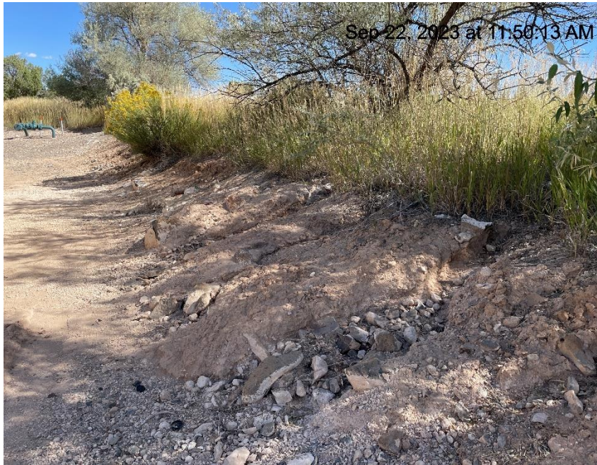
Photo # 364 Erosion & transport of sediment onto location/ insufficient BMP's
