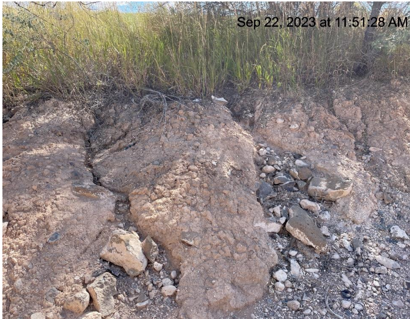
Photo # 386 Erosion & transport of sediment onto location/ insufficient BMP's
