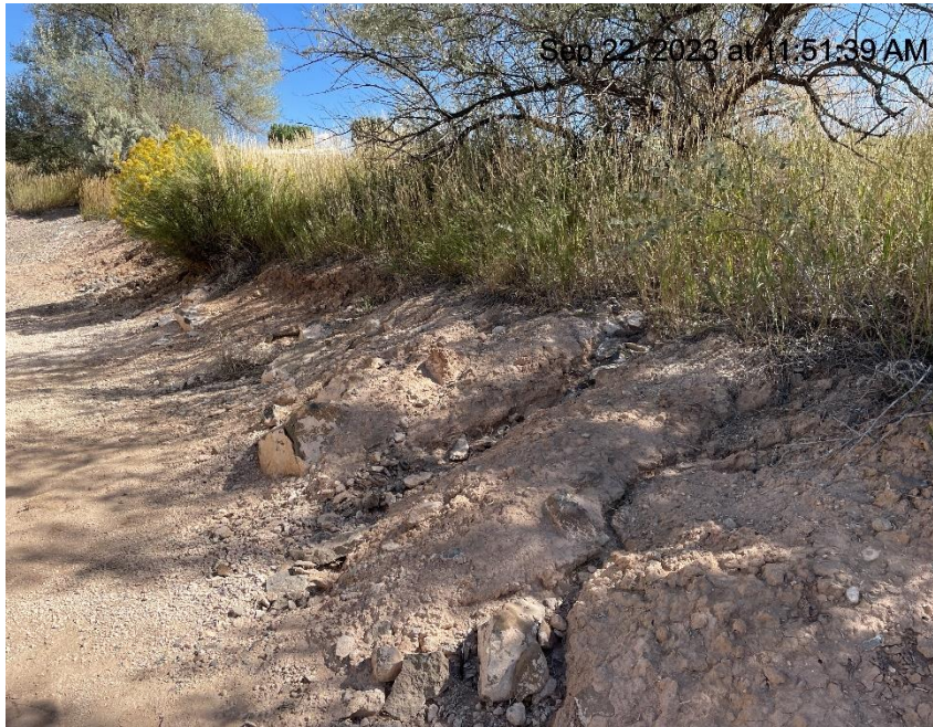
Photo # 389 Erosion & transport of sediment onto location/ insufficient BMP's
