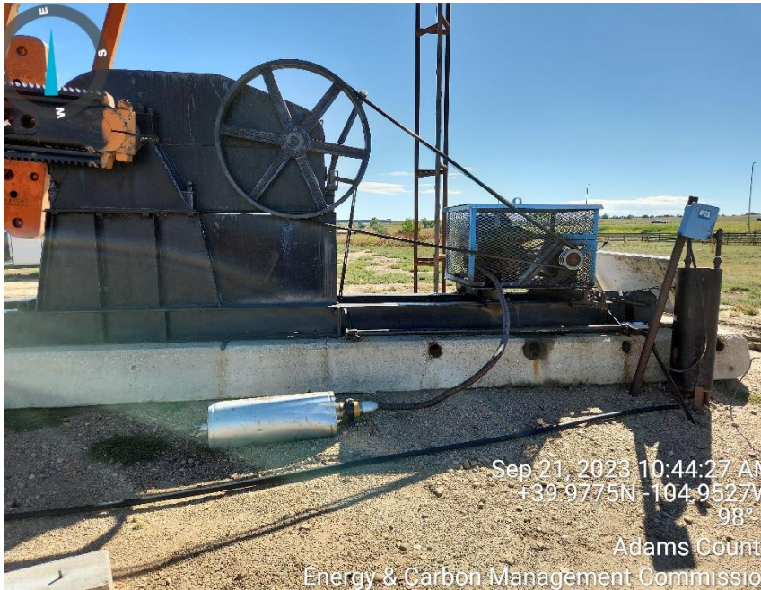
Photo 3 prime mover on pumping unit
