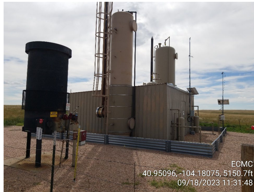
Photo 2 – ECD and Heater Treaters
