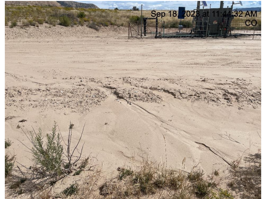
Photo # 9659 Erosion & transport of sediment into vegetated areas
