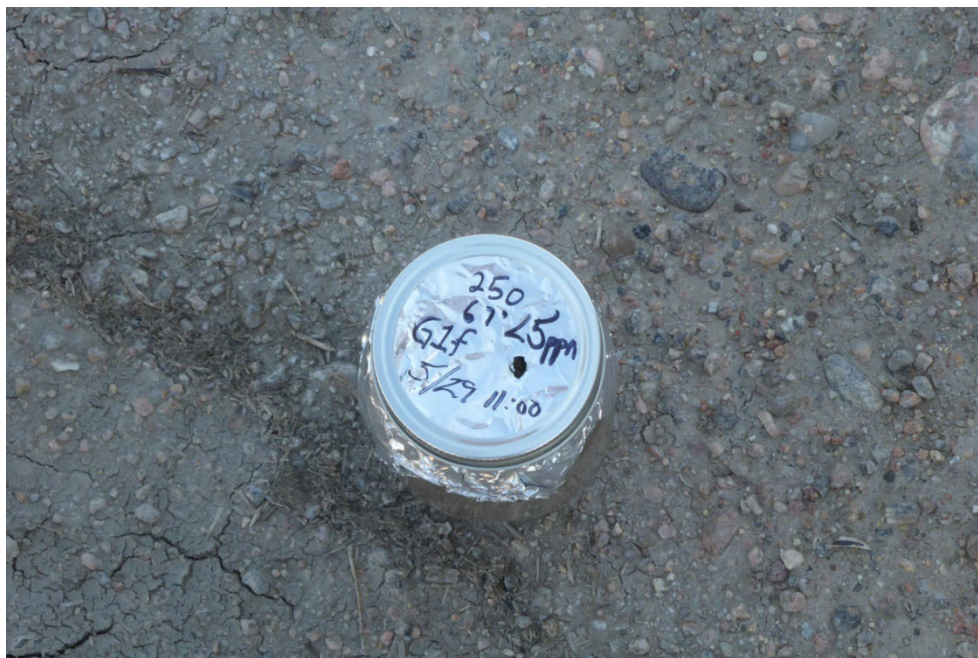
Field Sample G1f Located at the approximate mid-point of flowline ditch PID result <5 ppm from vapor space (after 30 minute heat cycle)
