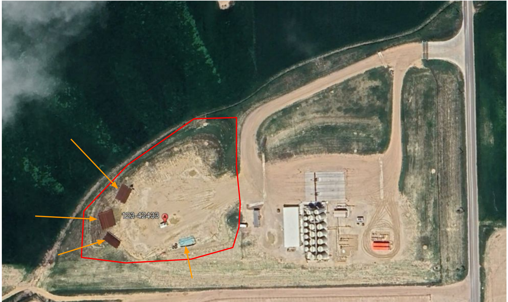
Photo 1. Google Earth aerial imagery from 5/24/2023 illustrating the location. Operator has failed to perform interim reclamation around the well location (red polygon) and is storing equipment (orange arrows) on the well location.
