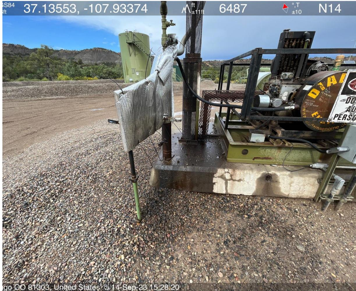
**Photo #4 View of impacted material on ground at muffler outlet.**
