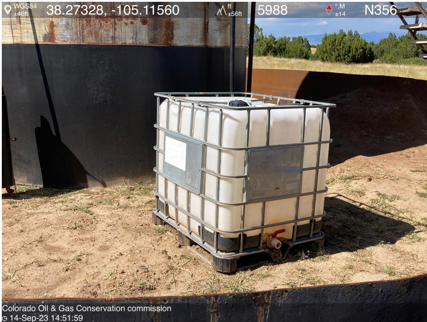
PHOTO 13: UNUSED EQUIPMENT STORED ON LOCATION (EMPTY LIQUID TOTE). REMOVE UNUSED EQUIPMENT PER RULE 606, IF TOTE IS NECESSARY FOR THE OPERATION OF THE WELL IT MUST BE LABELED. CA DATE 10-14-2023.
