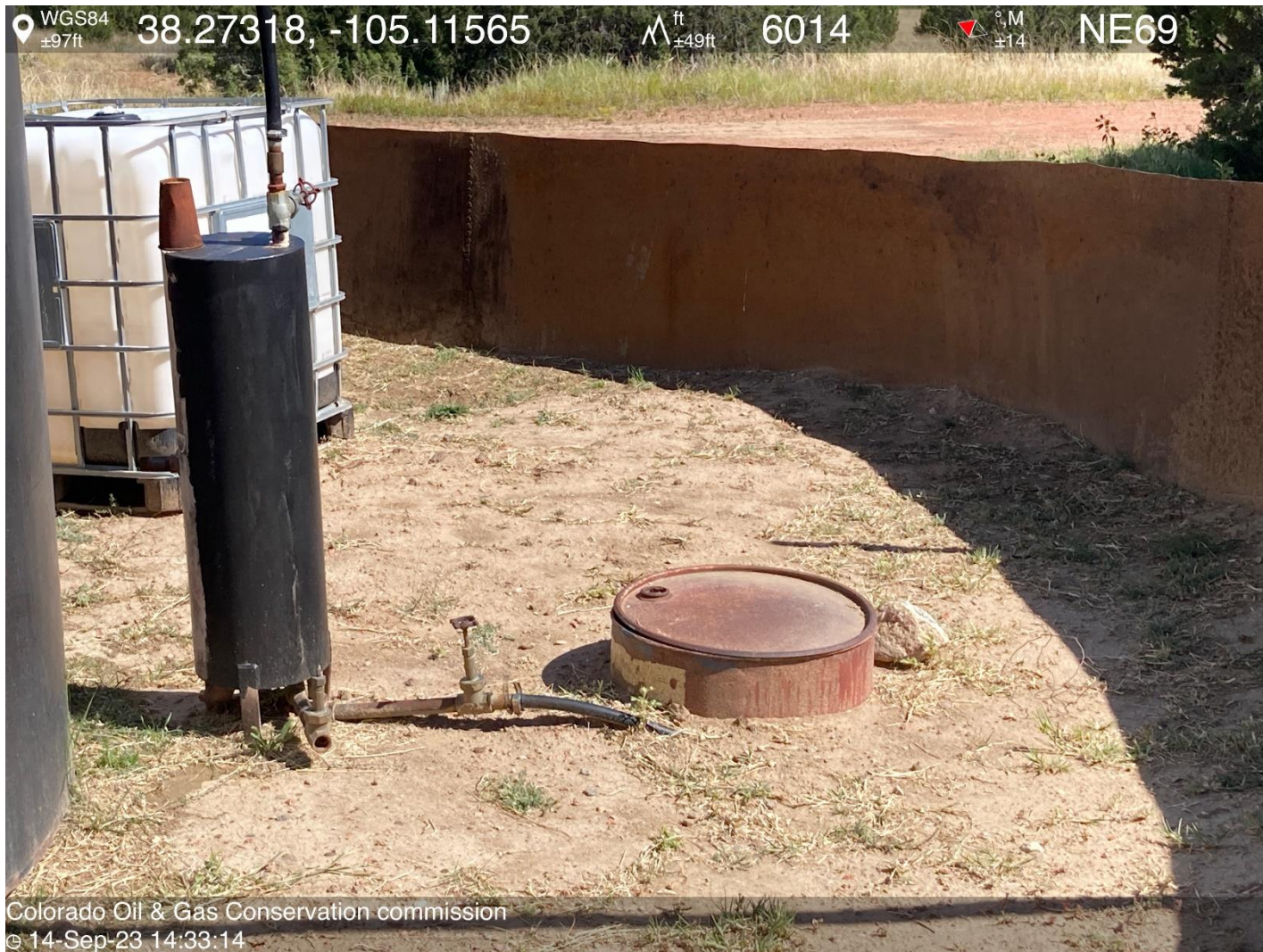
PHOTO 10: SEPARATOR IN LINE WITH 1" T-C ANNULUS SUPPLY LINE TO TANK BATTERY.
