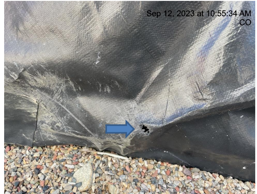
Photo # 8868 Hole in secondary containment liner/liner needs maintenance
