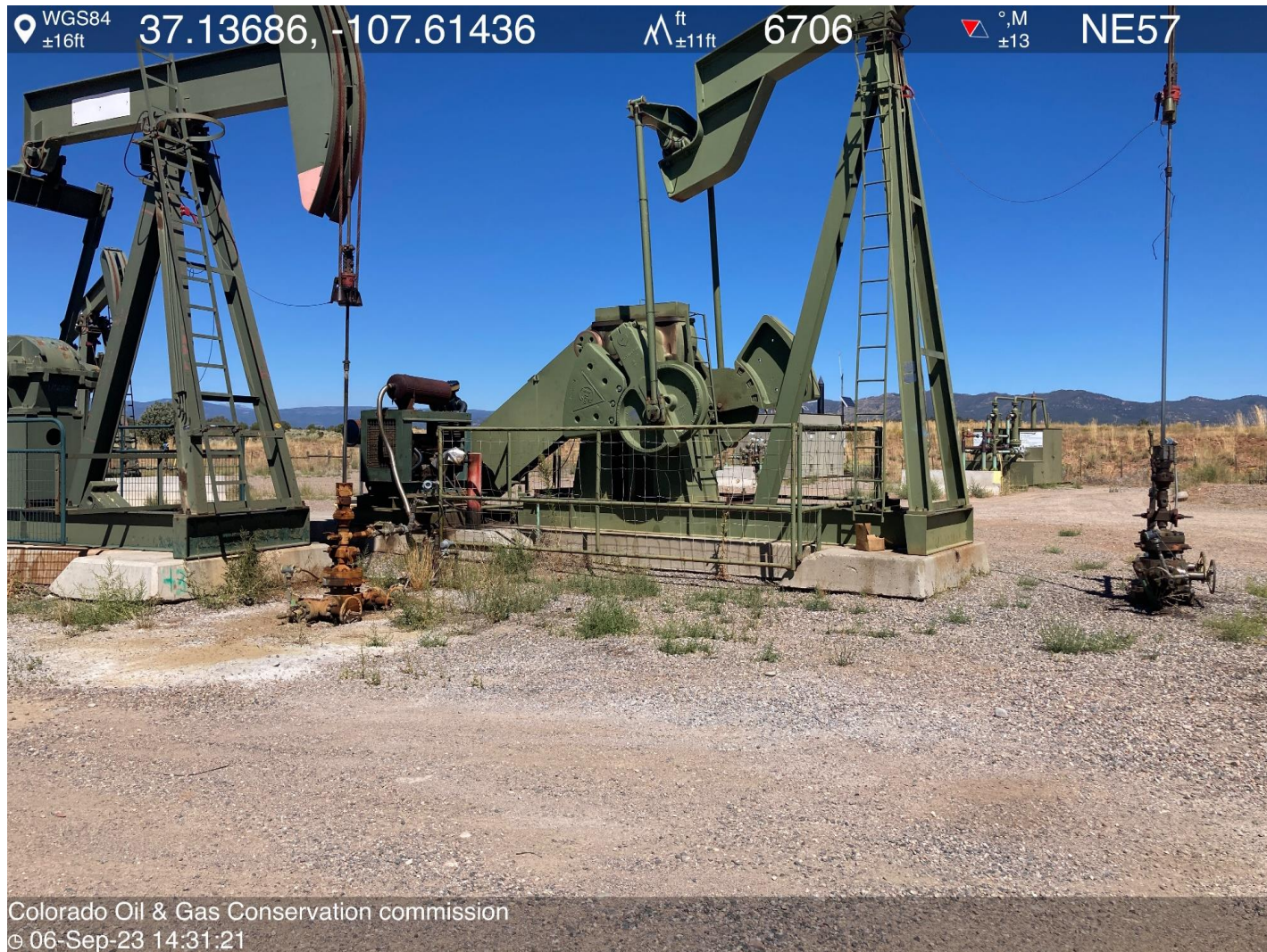
PHOTO 4: WELLHEAD AND EQUIPMENT. NO WELL SIGN IDENTIFYING EACH WELL. POST SIGN PER RULE 605 10-6-2023.
