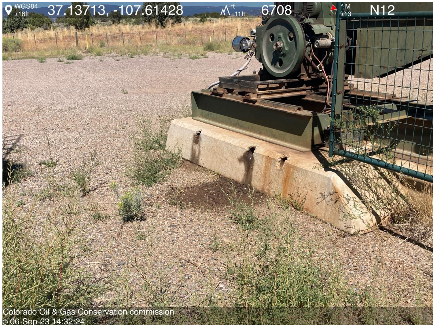
PHOTO 11: Oily waste appears to be from pump jack prime mover is impacting soil near prime mover. Securely fasten all valves, pipes, fittings, and Production Facilities to ensure good mechanical condition, inspect at regular intervals and maintain in good mechanical condition and dispose of impacted materials per Rule 608.e. ca date 10-6-2023.
