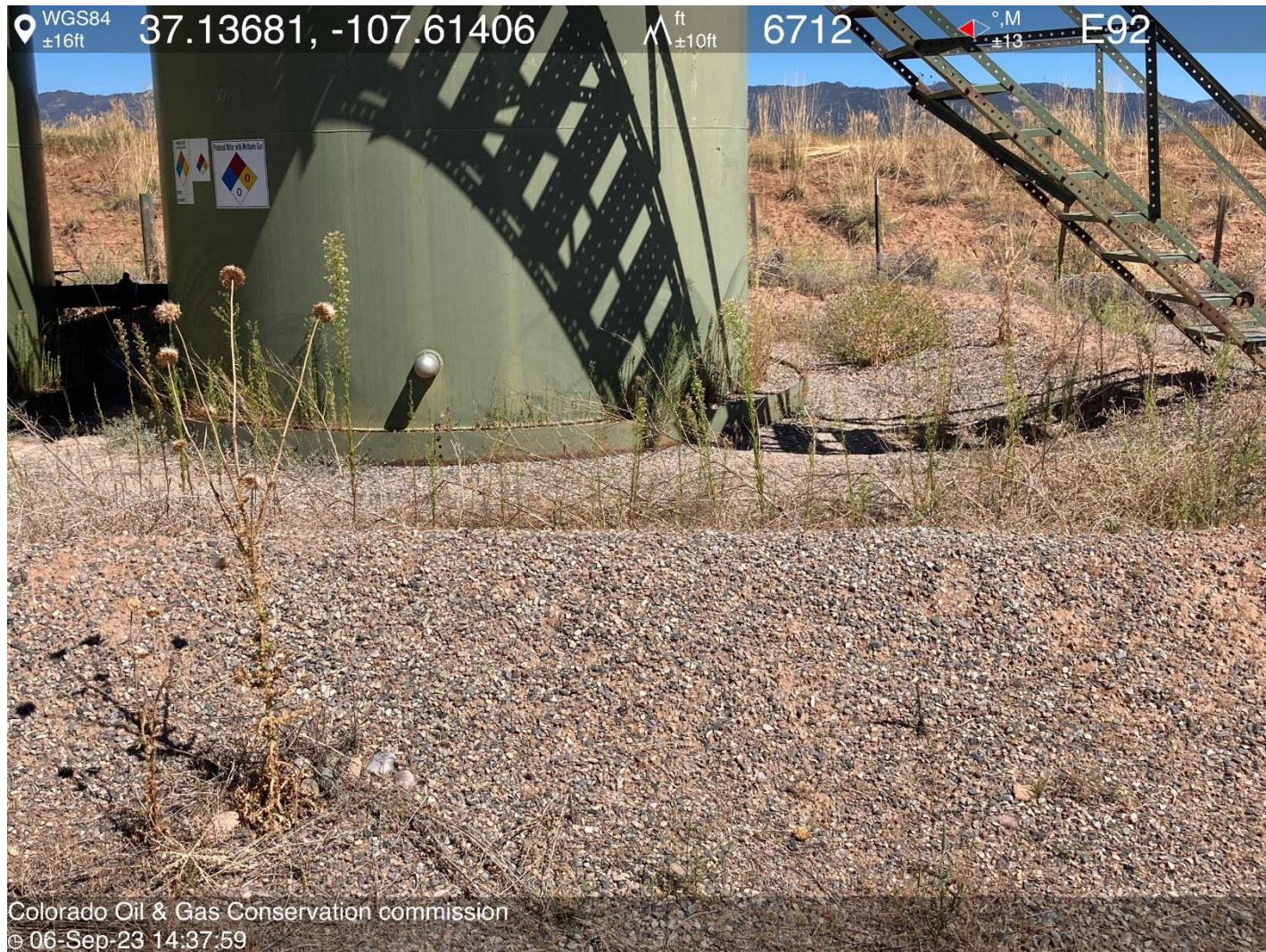
PHOTO 13: Tall weeds on and inside berms. Maintain berms/ remove weeds along with there root structures per rule 605.a. ca date 10-6-2023.
