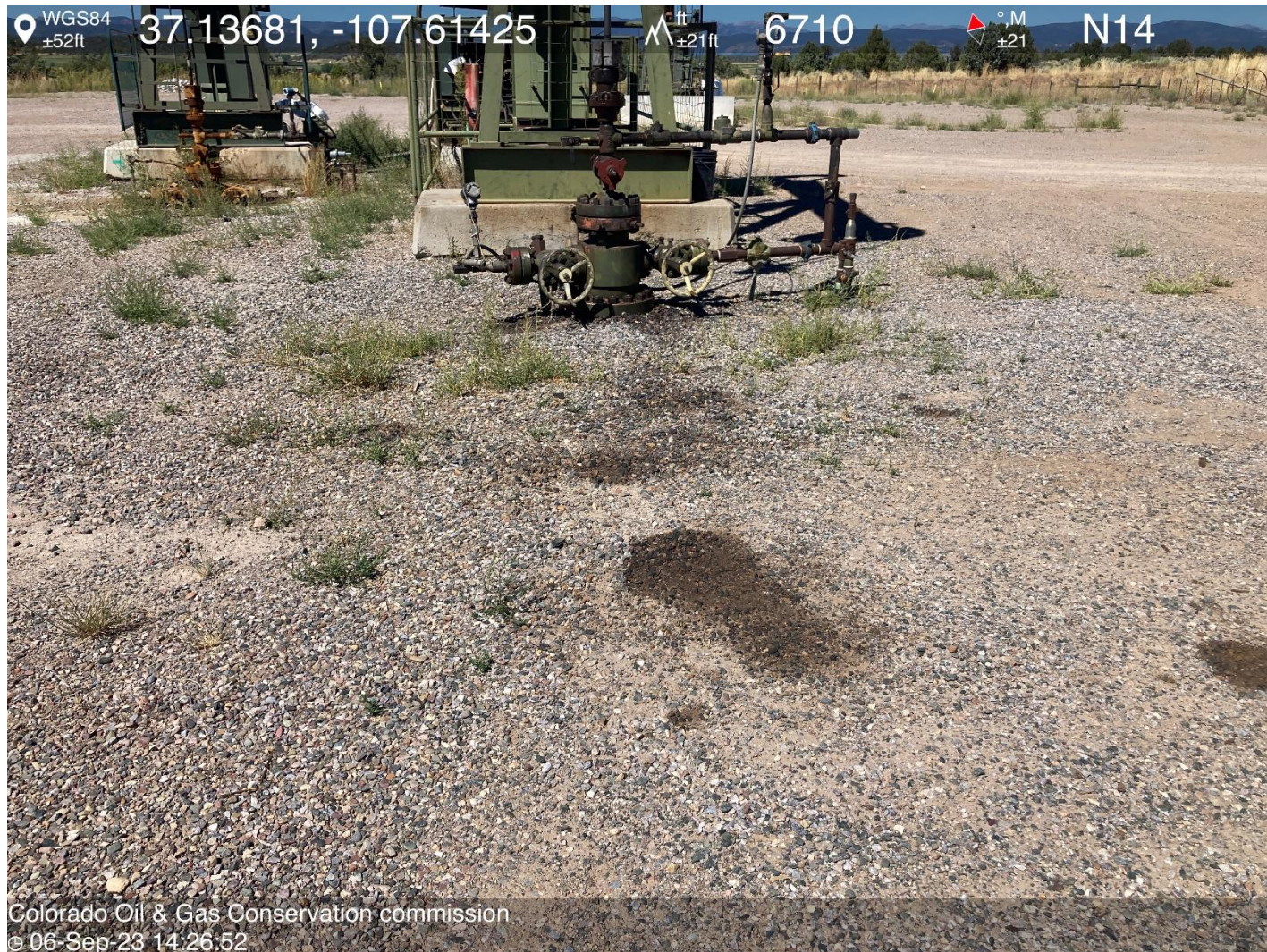
PHOTO 10: Oily waste appears to be from rod box impacting soil near wellhead. Securely fasten all valves, pipes, fittings, and Production Facilities to ensure good mechanical condition, inspect at regular intervals and maintain in good mechanical condition and dispose of impacted materials per Rule 608.e. ca date 10-6-2023.
