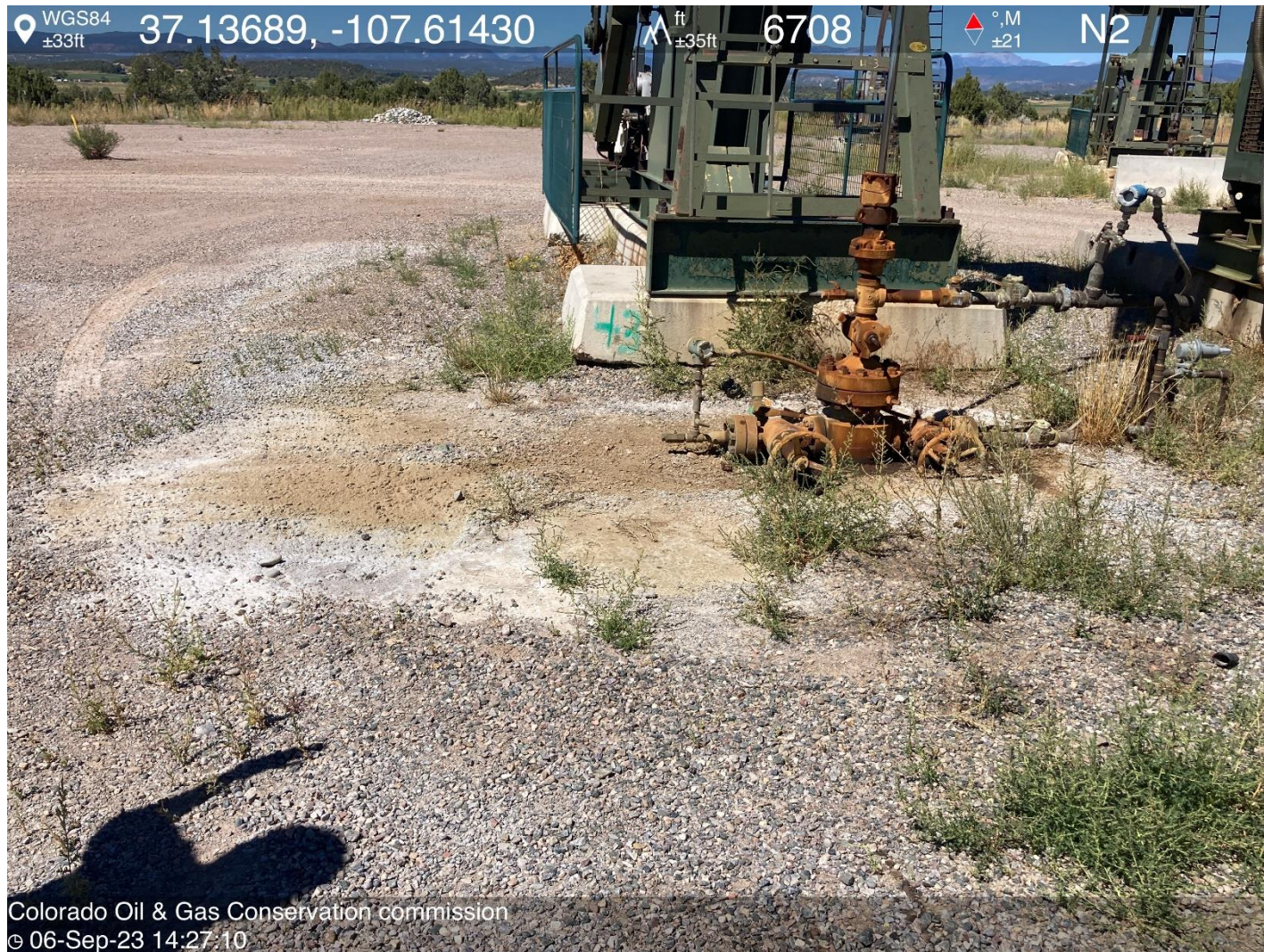
PHOTO 9: Produced water spill from the wellhead has left a salt/mineral impacted area around the wellhead. Securely fasten all valves, pipes, fittings, and Production Facilities to ensure good mechanical condition, inspect at regular intervals and maintain in good mechanical condition and dispose of impacted materials per Rule 608.e. ca date 10-6-2023.
