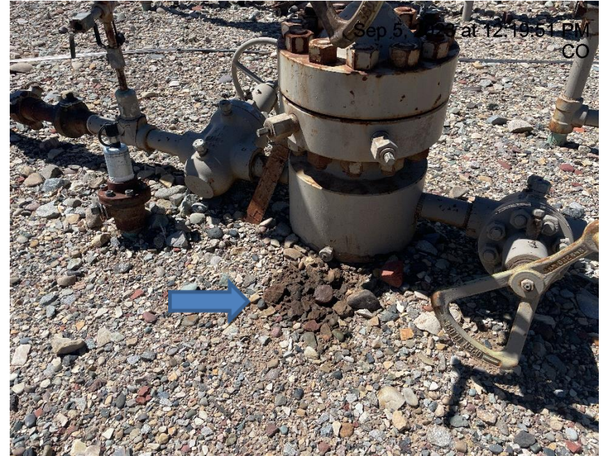
Photo # 8241 Stained soils & gravel near wellheads
