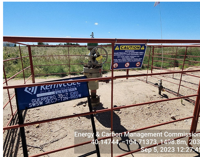
Photo 2: TA Wellhead
