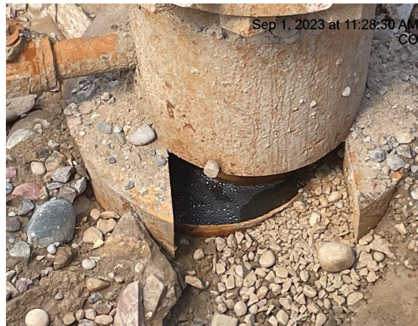
Photo # 8050 MCU 26-4A well, gas is bubbling up from conductor
