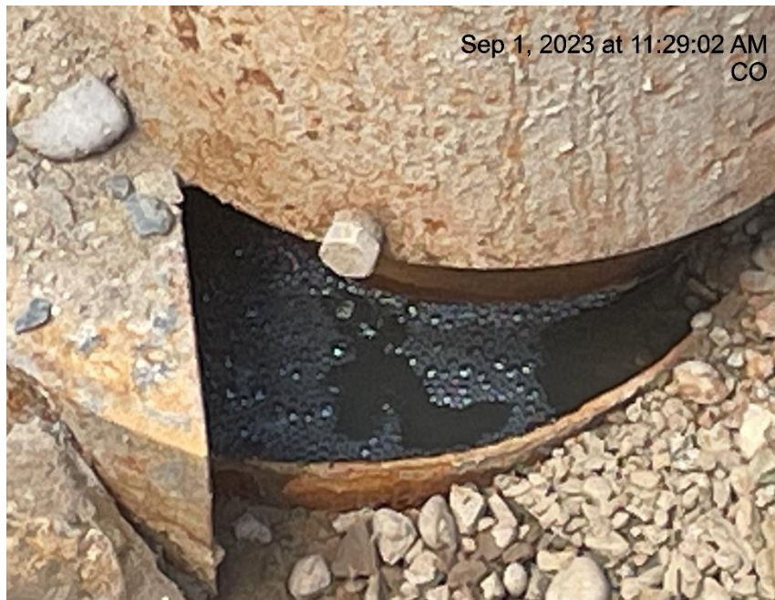
Photo # 8055 MCU 26-4A well, gas is bubbling up from conductor
