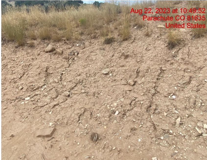
Insufficient Erosion Control/Rill Erosion Running Onto Location – Photo #06023
