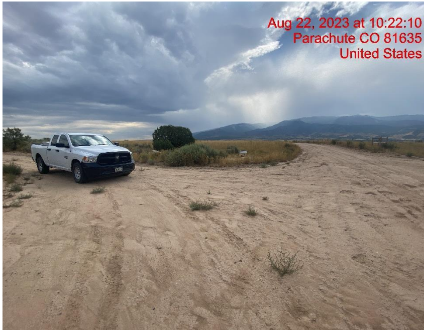
Insufficient Vehicle Tracking BMPs at Location Entrance/Exit – Photo #06014
