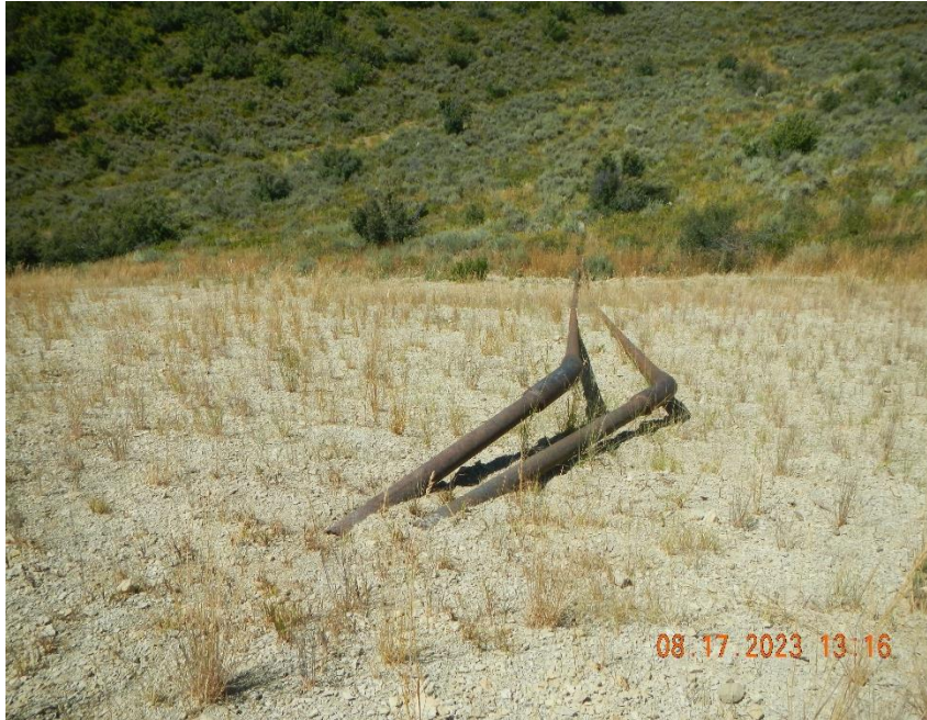
2 – 4" unused flowlines at north west edge of location
