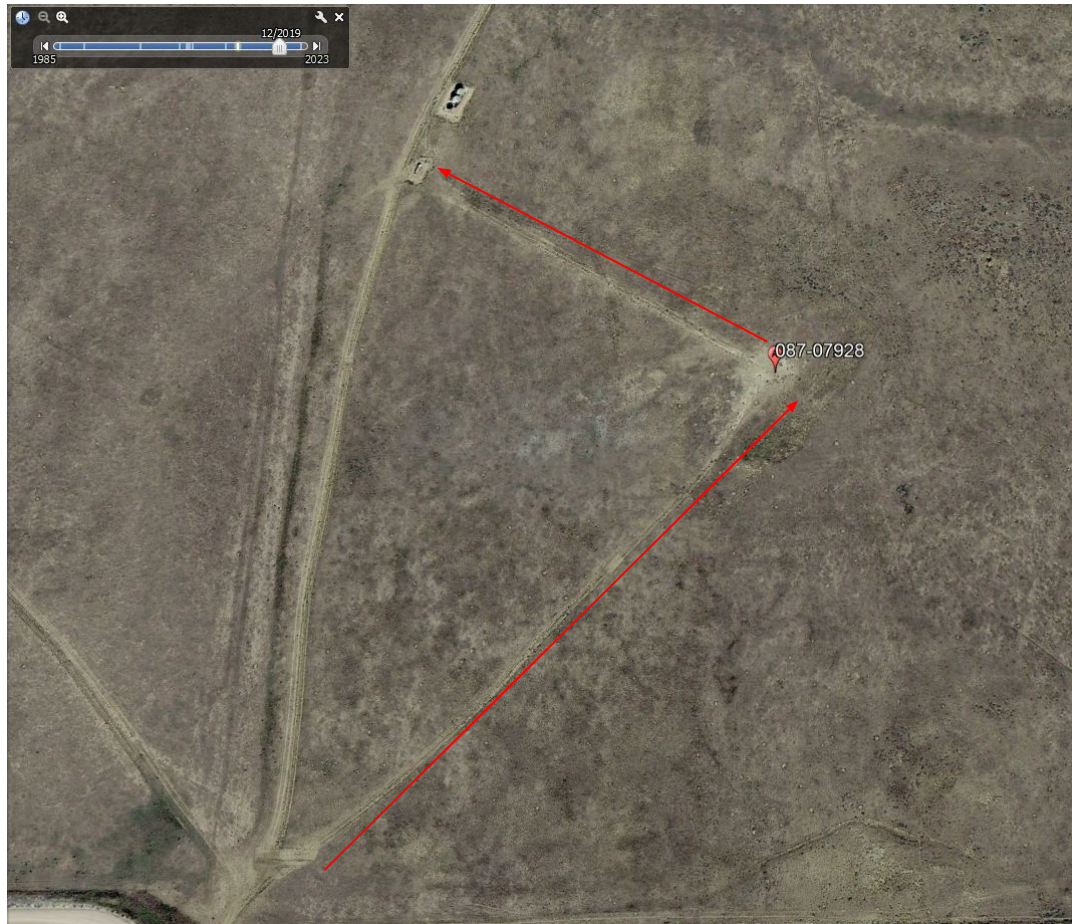
Photo 8. Google Earth aerial imagery taken circa 12/2019. Photo illustrates the access roads that require additional reclamation activities to comply with Rule 1004. During this inspection, Staff walked both access roads and observed that re-grading and contouring is required as heavy rutting (as deep as 1') was evident.
