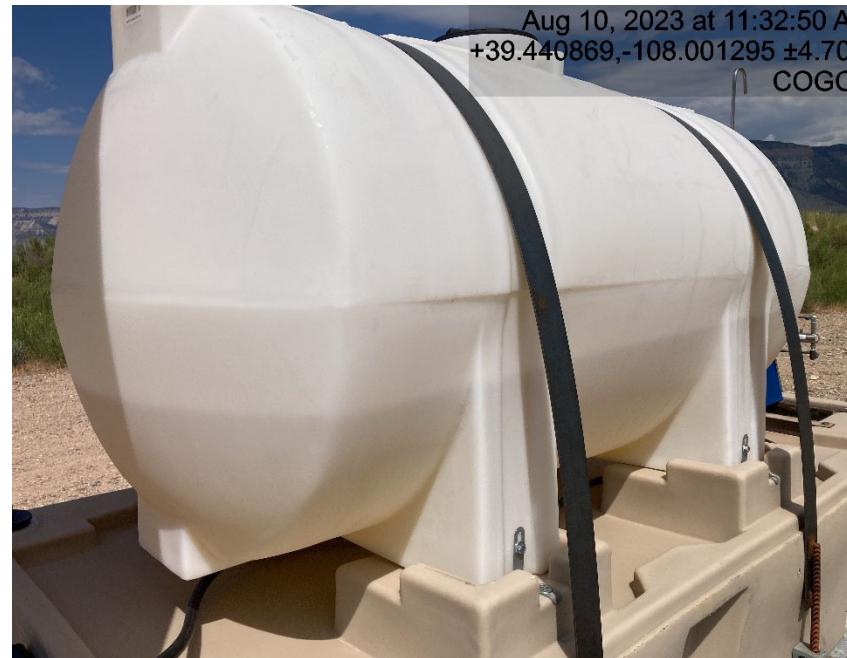
Tank lacking labeling
