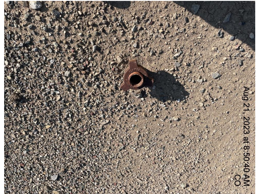
Photo # 6630 Open ended piping/wildlife hazard
