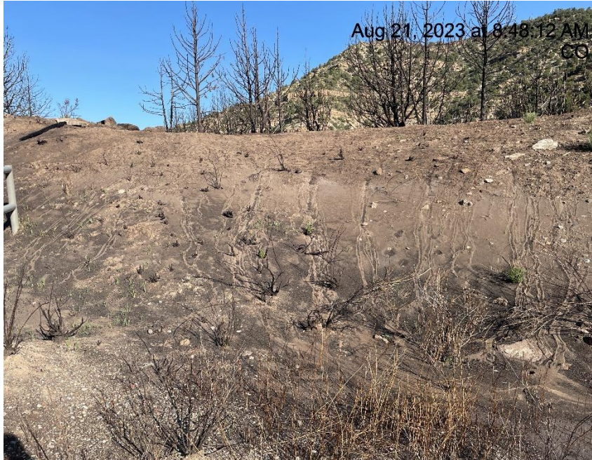
Photo # 6621 Erosion & transport of sediment (N/NE area of location on slope near wellheads)
